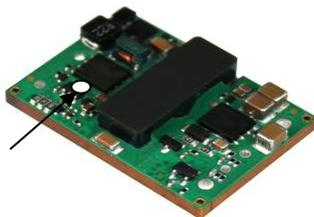
Location of heatless substrate test points
